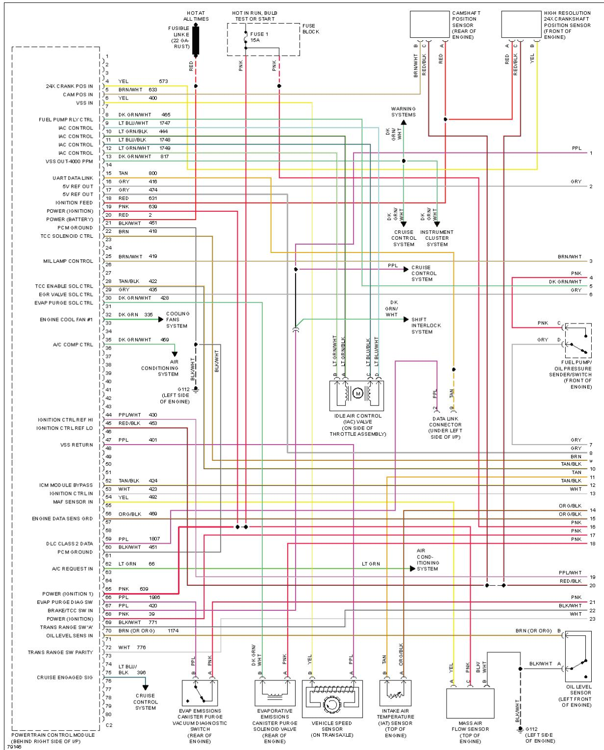
Fig. 10: 3.1L (VIN M), Engine Performance Circuits (1 of 3)
