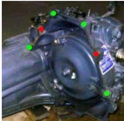
Transmission Bolt Placement.
